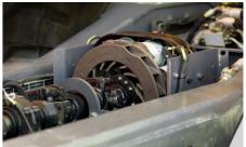
In applications with a high degree of downhill tramming, the retarder, integrated in the control system, provides wear free braking and retardation via electromagnetic induction.
