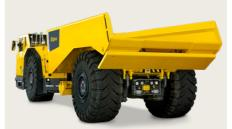
Available engine alternative are the EPA Tier The smart, hydraulically operated tailgate works as a spill guard and supports the filling process with one extra side in the box.
